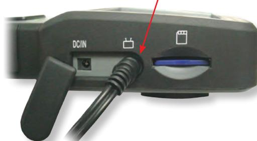
The video output format to the auxiliary display may be switched between NTSC and PAL by using the VIDEO FORMAT function on the main menu.
