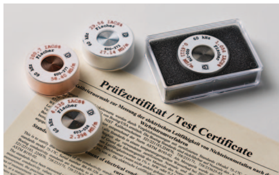
Certified standards for calibrating the SIGMASCOPE® SMP350, traceable to internationally-recognised calibration norms
