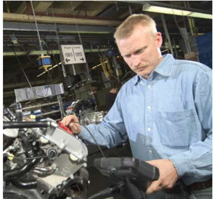
Inspect valve seating through the spark plug port
