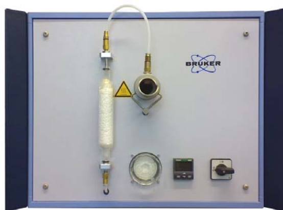
Figure 4: Front panel of the ICARUS TF furnace module.
