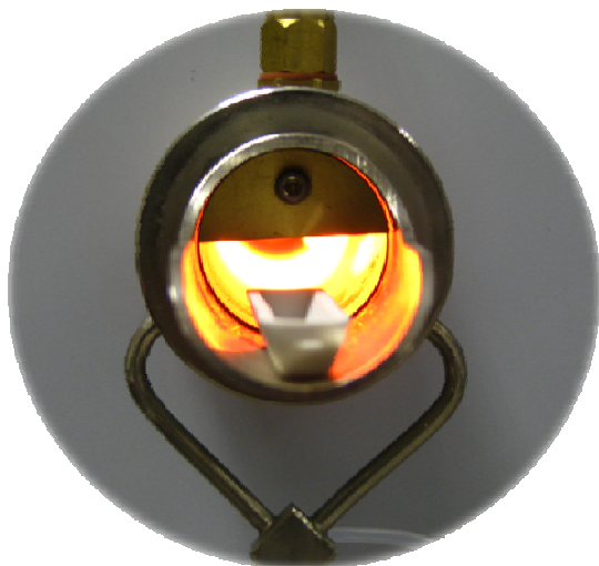
Figure 5: End-on view of the tube furnace and combustion boat.
