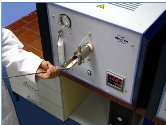
Figure 2: Sample and ceramic boat being inserted into the furnace of the ICARUS TF.
