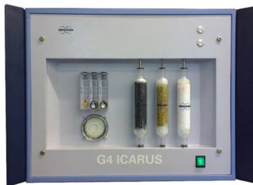
Figure 6: Front panel of the ICARUS TF analyzer module.
