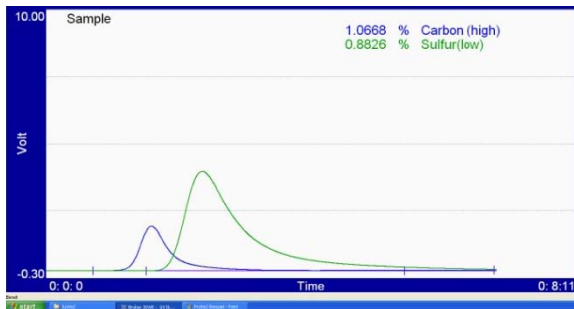
Figure 7: Carbon (blue) and sulfur (green) temporal peak profiles from a single analysis of cement.
