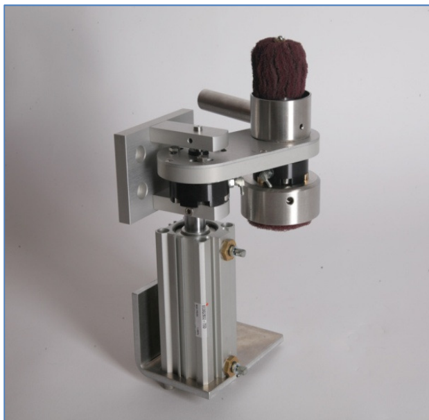
Figure 7. Dual-brush system for automatically cleaning the electrodes in the G8 GALILEO ON/H (vacuum cleaner and integrated hose system not shown).
