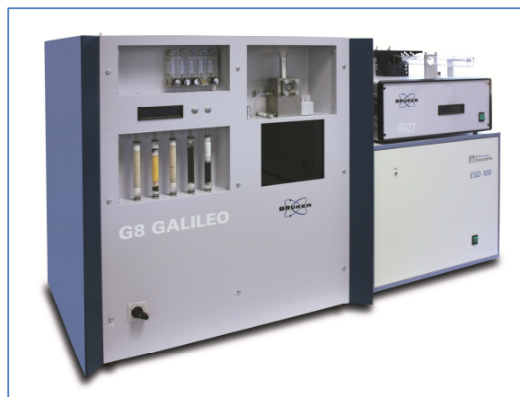
Figure 9. G8 GALILEO ON/H with external diffusible hydrogen module (upper right) and commercial mass spectrometer (lower right).
